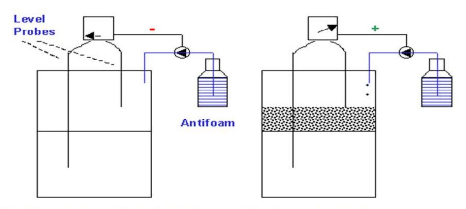
When the upper level probe is above the foam level, no current will pass between the level probes and the antifoam pump remains turned off.
