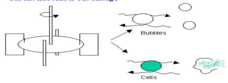
With radial flow impellers, vertical (or axial) mixing is achieved with the use of baffles
