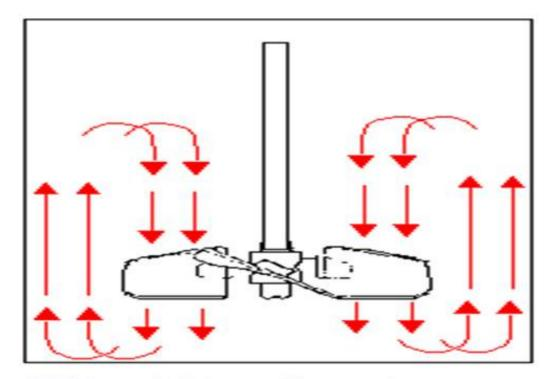
With axial impellers, the liquid is pushed in a downward direction; that is, along the axis of the reactor.
