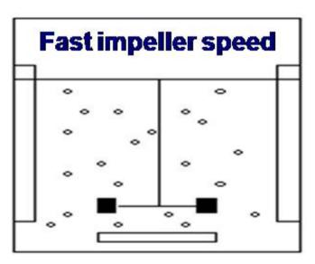
Smaller bubbles will be generated and these bubbles will move with throughout the reactor increasing the gas hold up and bubble residence time
