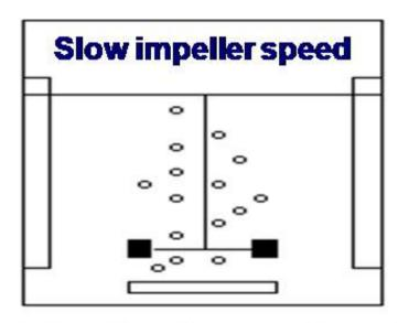
The bubbles will not be sheared into smaller bubbles and will tend to rise directly towards the surface
